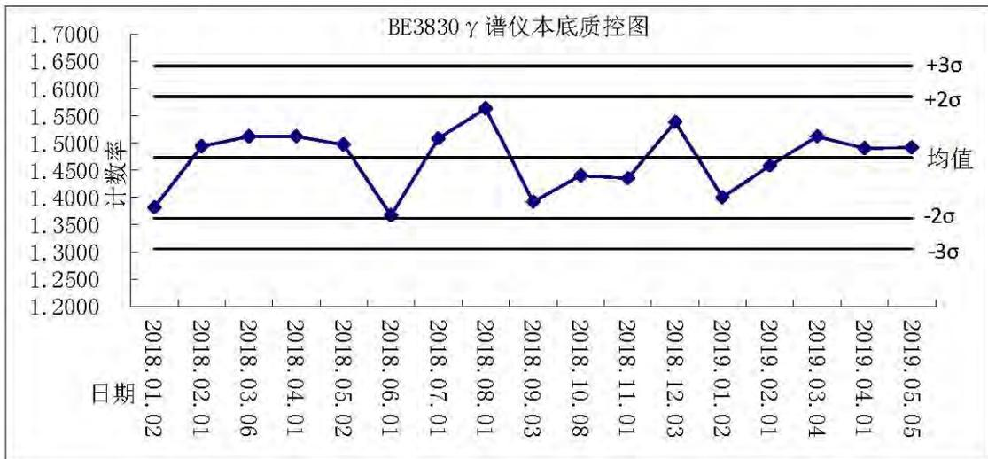
图 3.1-8 BE3830 $\gamma$  谱仪本底质控图
